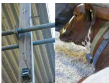
The receiver registers the movements of animals equipped with a neckband for activity measurement.
